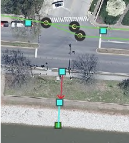
2016 Kanawha Blvd, 10 VCP, 50 LF (2' sect. repair by City St. Dept.)
