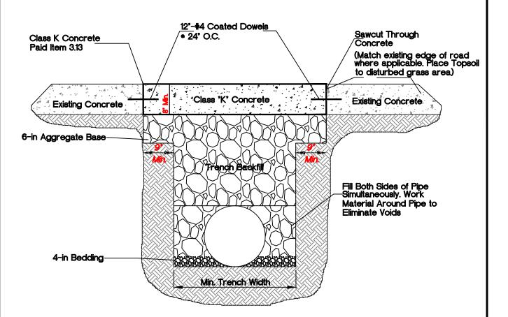
Match existing edge of pavement where applicable City shall direct limits of Class K Concrete. Use 1/2' dia. epoxy coated dowel, 12' long, 24' on-center if existing concrete street is 6' thick or greater. or greater.
