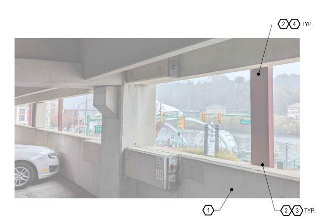
2. VERIFY LOCATION OF POSSIBLE ELECTRICAL CONDUIT IN HOLLOW METAL FACADE COLUMNS PRIOR
